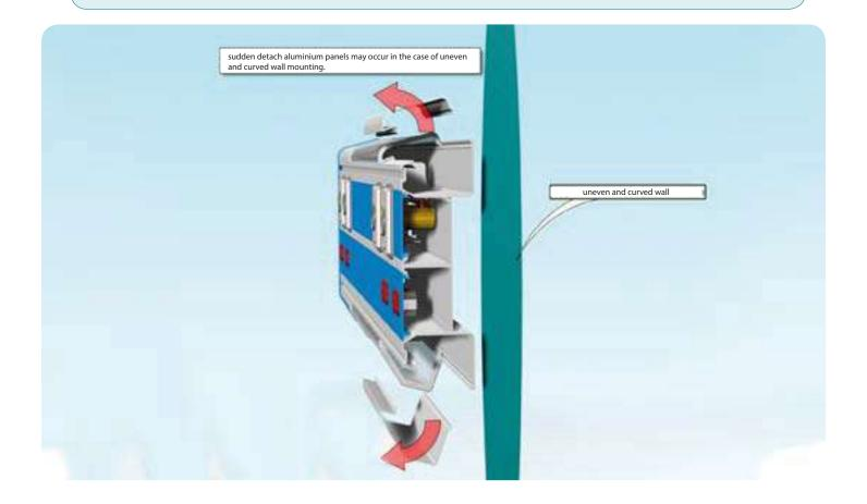
Verify that the structure is not deformed due to an excess of torque in the fixing screws, in case of an excess of torque, the structure of the medical horizontal headwall will present deformation.
