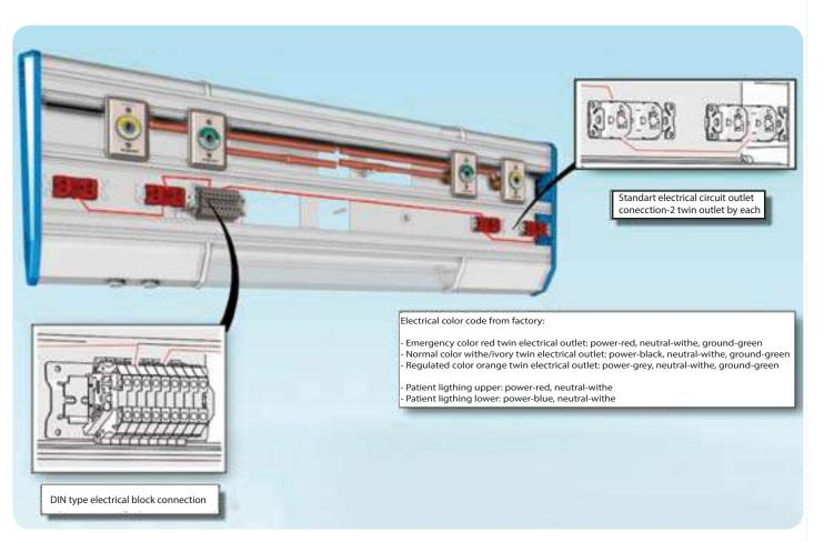
Will be specify from the factory to 127V 20A, a different voltage type and electrical wire size will be noticed to the factory in advance.
