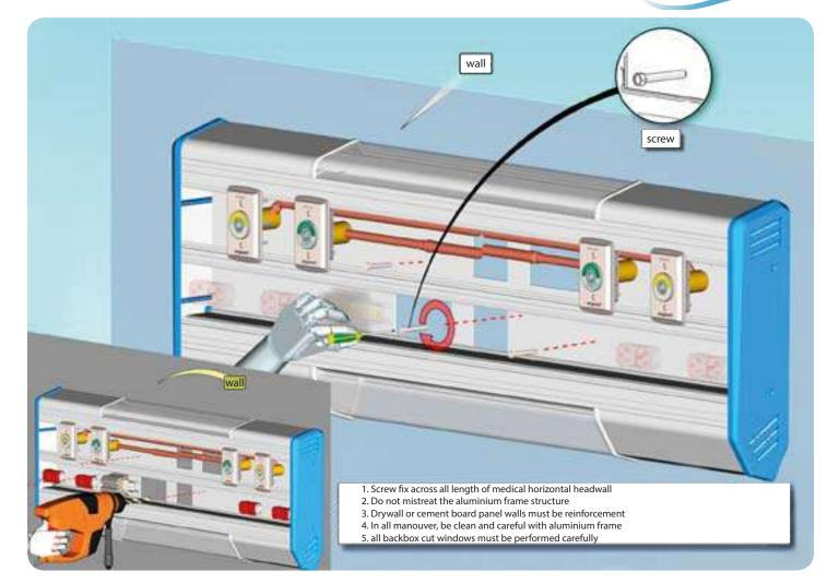
Once the medical horizontal headwall be fixed on the wall, proceed to connect all electrical, lighling, medical gases, voice and data systems.
