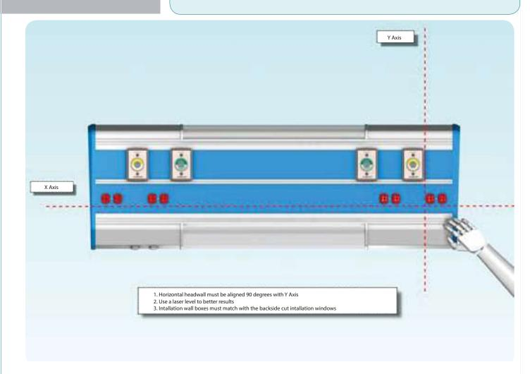
Without the front panels installed, you must proceed to position on the wall, match with the wall installation back boxes and in a correct alignment on the "Y" and "Z" axes (vertical and horizontal), proceed to the fixing with screws.
